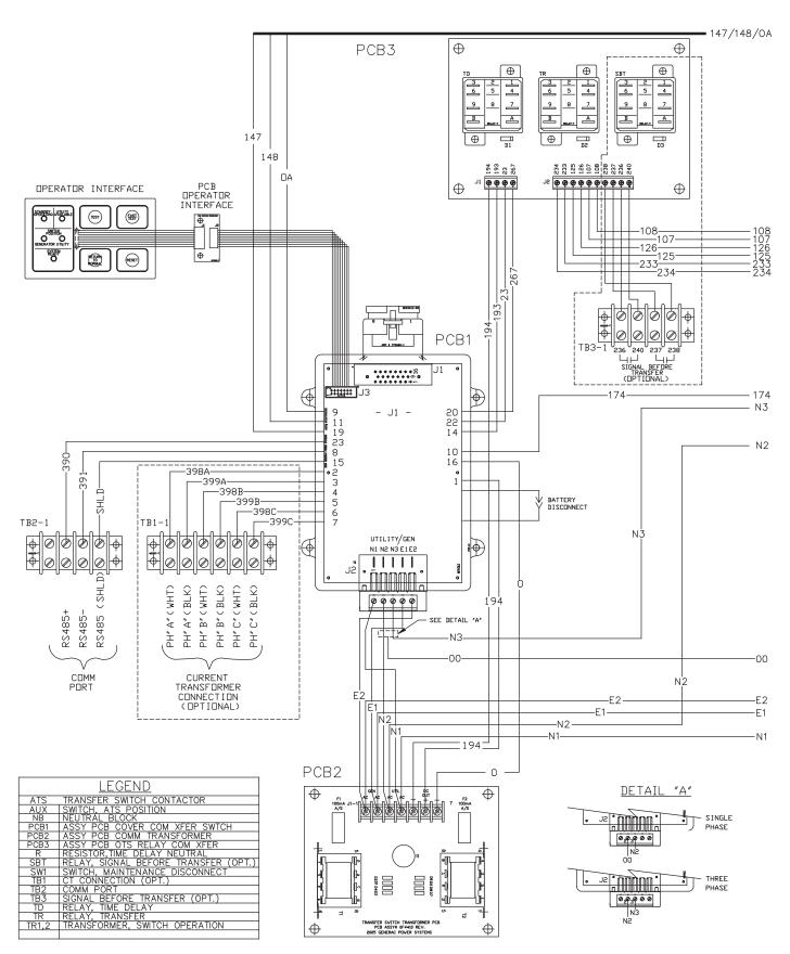
Wiring Diagram - 208/240V — Drawing No. 0F7043-B
