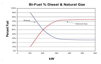
Only slightly more expensive than diesel-only designs, bi-fuel generators offer several important advantages. For one, the lower capital cost of a compression-ignited engine is retained while capitalizing on many of the advantages of gaseous fuel, such as
